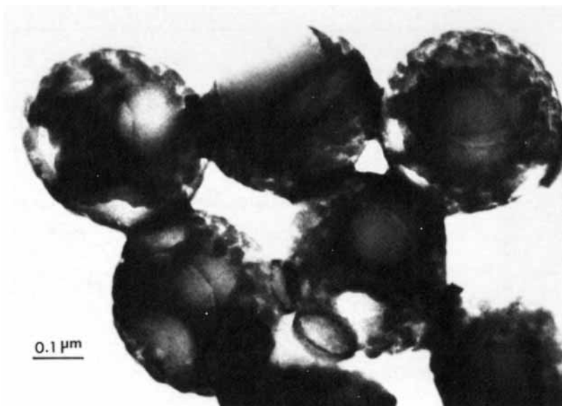
Figure 4 TEM of PS300/PEMA-AIBN composite polymer particle with 40/60 weight seed to shell ratio. Dark regions are polystyrene stained with RuO 4 and lighter regions are acrylate domains outlined using phosphotungstic acid stain.
